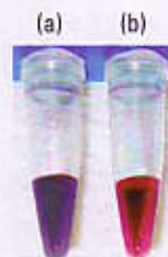
(a) A blue-gray color indicates that a control probe is bound to DNA. (b) A pink color indicates that a mismatched probe has melted off the SNP-containing DNA.
